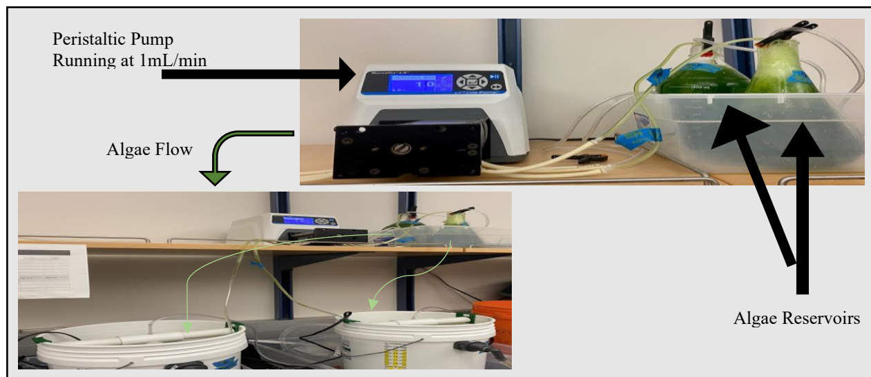
Figure 1. Peristaltic Pump and Algae Reservoirs. Tubing connects the algae reservoirs to the rotifer culture buckets at a rate of 1ml/min via peristaltic pump.
