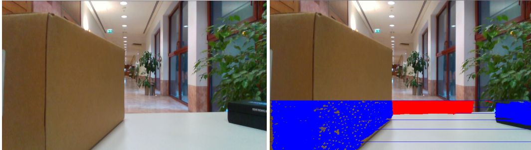
Figure 3.6: Depth Anomaly Detection Example
