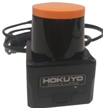
Figure 3.2: Hokuyo UST-10LX LiDAR
