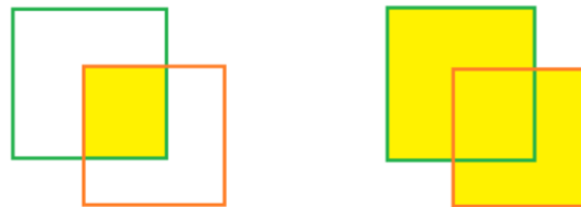
Figure 2.6: IoU. Green boxes mean bounding boxes of ground truth. Red boxes are the prediction results. (Left) The area of overlap. (Right) The area of union.
