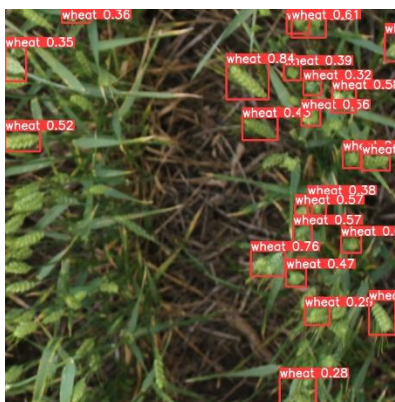
Figure 3.9: The detection example of low-resolution images in GWHD_2021 dataset with a 50-epoch trained YOLOv5 model.
