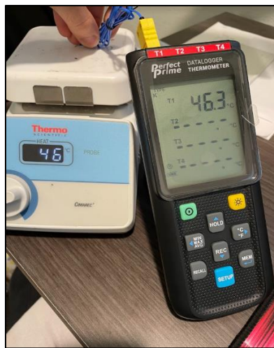
Figure 2.14: Heating Element Functional Test
