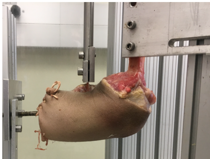
Figure 2.15: Specimen locked at 90° flexion for ramp testing.
