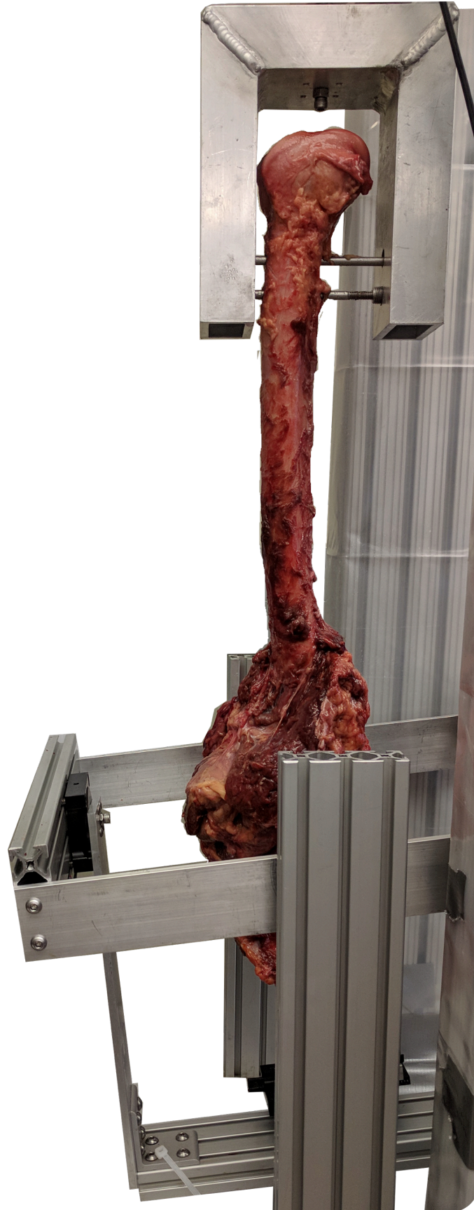
Figure B.4: Hip sample loaded in reconfigurable testing machine
