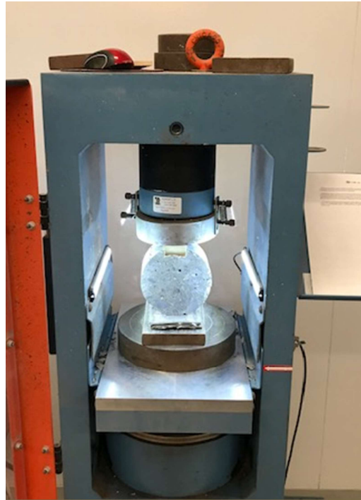
Figure 7.4 Splitting tensile strength test setup
