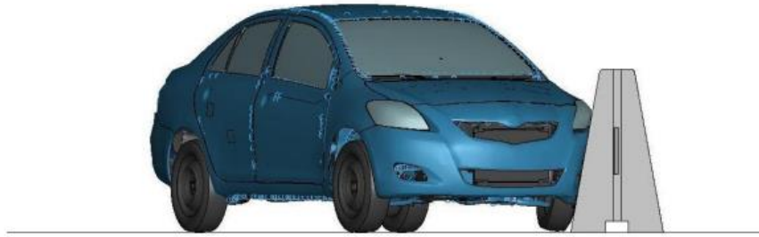
t = 0.10 s, event = front right tire contacts the barrier
