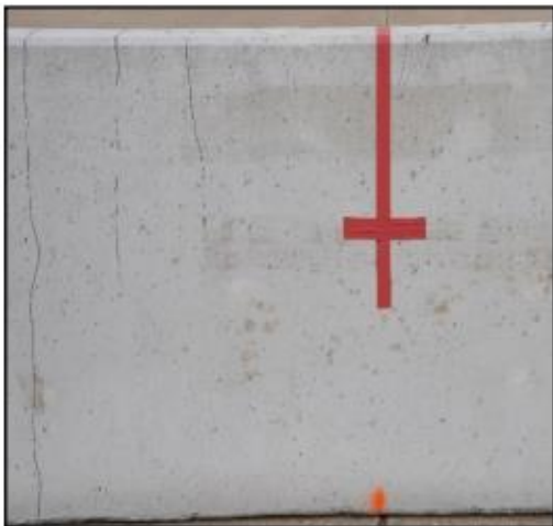
Figure 16. Damage observed on the impact side the single slope barrier after the component testing performed to evaluate the barrier strength.
