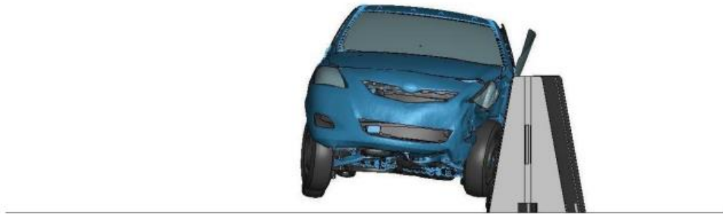
t = 0.23 s, event = rear right tire contacts the barrier, windowpane snags against the barrier
