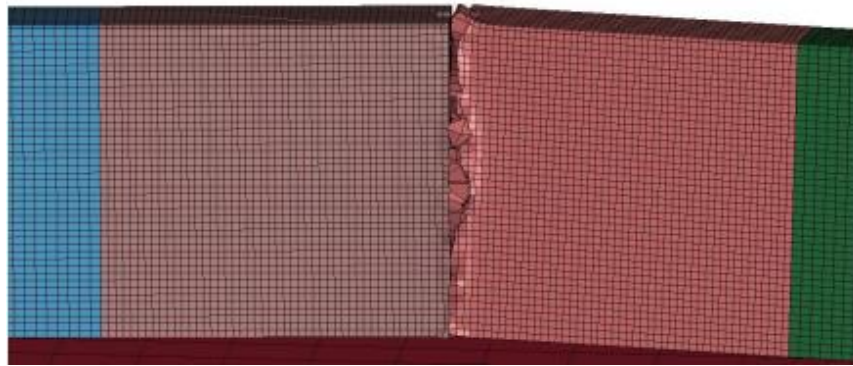
Figure 101. Single slope barrier simulation without hourglass card
