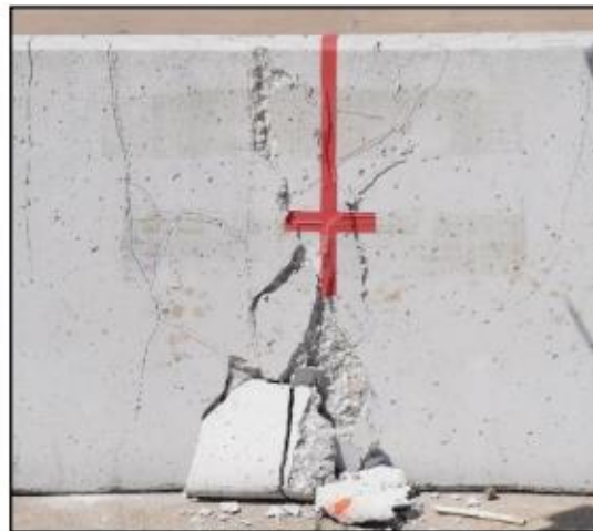
Figure 16. Damage observed on the impact side the single slope barrier after the component testing performed to evaluate the barrier strength.
