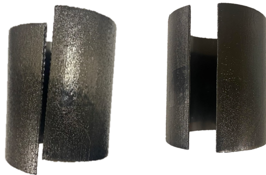
Figure 36: Original balanced layup [90/45/0/-45/90] on left, twinned layup on right
