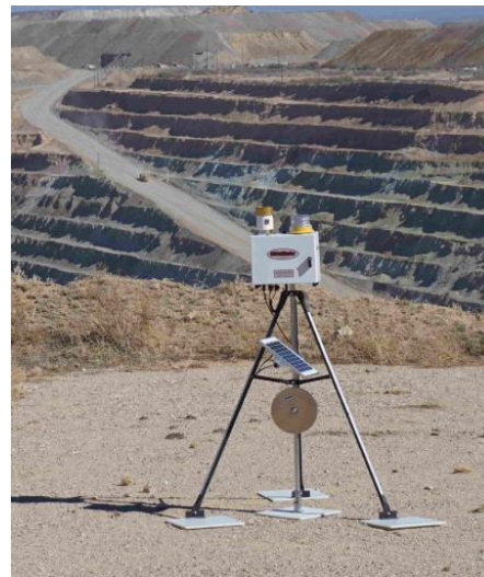
Figure 2.17 Wireline extensometer (photo from a public source https://www.cnitucson.com/ )
