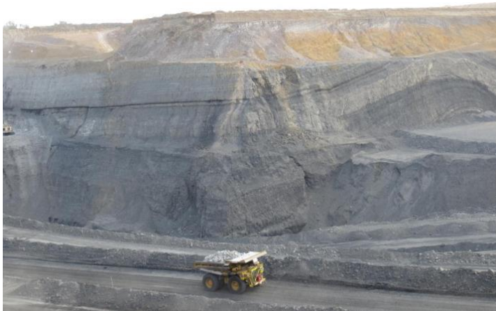
Figure 5.1 Convex shape of the pit wall. This “nose” shape is less stable than plane strain wall (reprinted from McQuillan et al. 2018)
