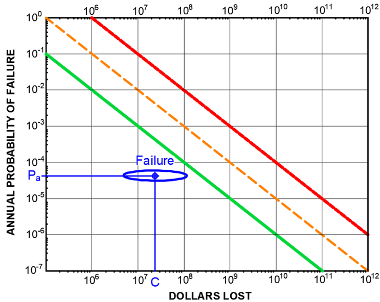
Figure 3.77 Example of the risk chart; the location of the activity has coordinates of P_a and C .
