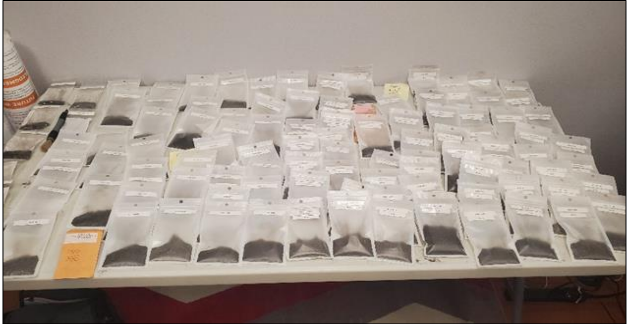
Figure 5: Cuttings after they were transferred into resealable sample bags to reduce further sample degradation due to evaporation. Bags are labeled to include depth interval, mass, formation tops, and flags for possible contamination.
