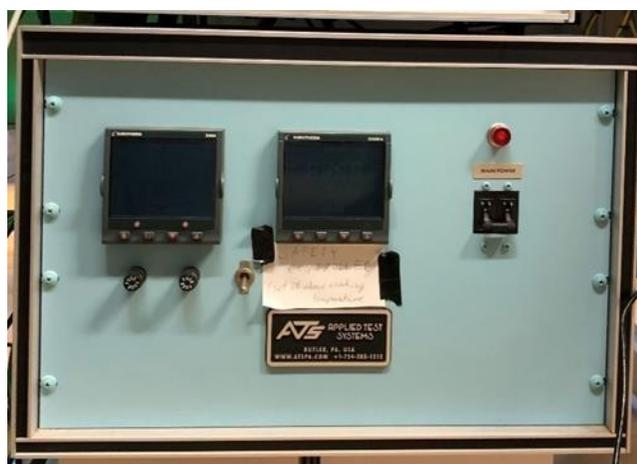
**Figure 24: Temperature controller**
