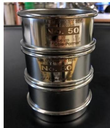
Figure 30: Sieves of sizes 300 and 425 $\mu$ m
