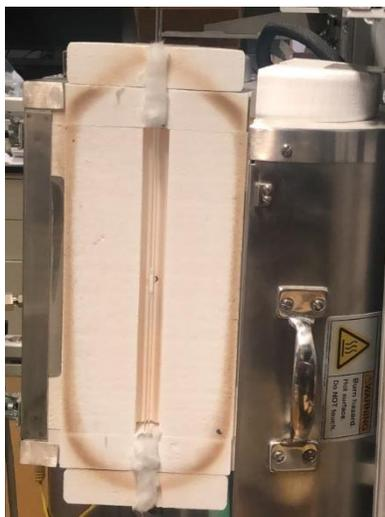
**Figure 31: Loaded reactor inserted into the furnace**
