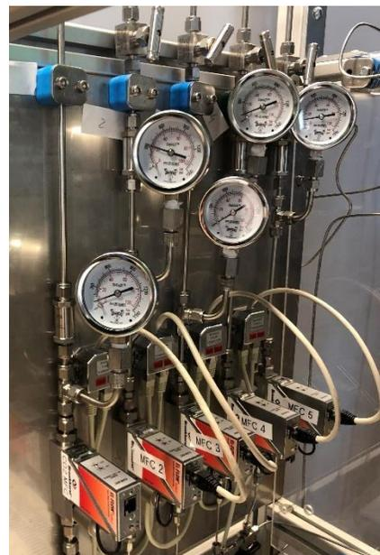
**Figure 23: Mass flow controllers and pressure indicators**
