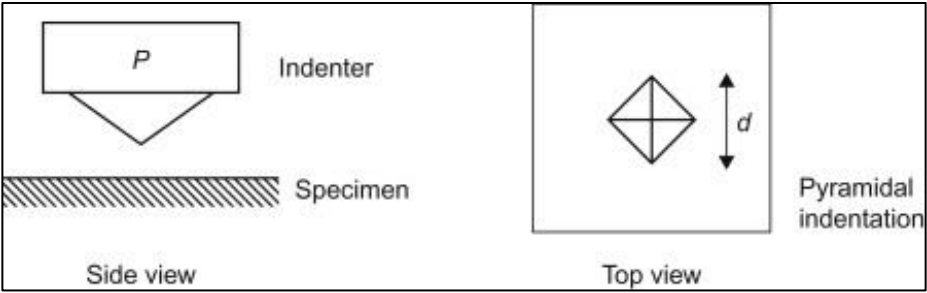
Figure 21: Indenter and indentation made for the microhardness measurements. Adapted from Smallman and Ngan [157]
