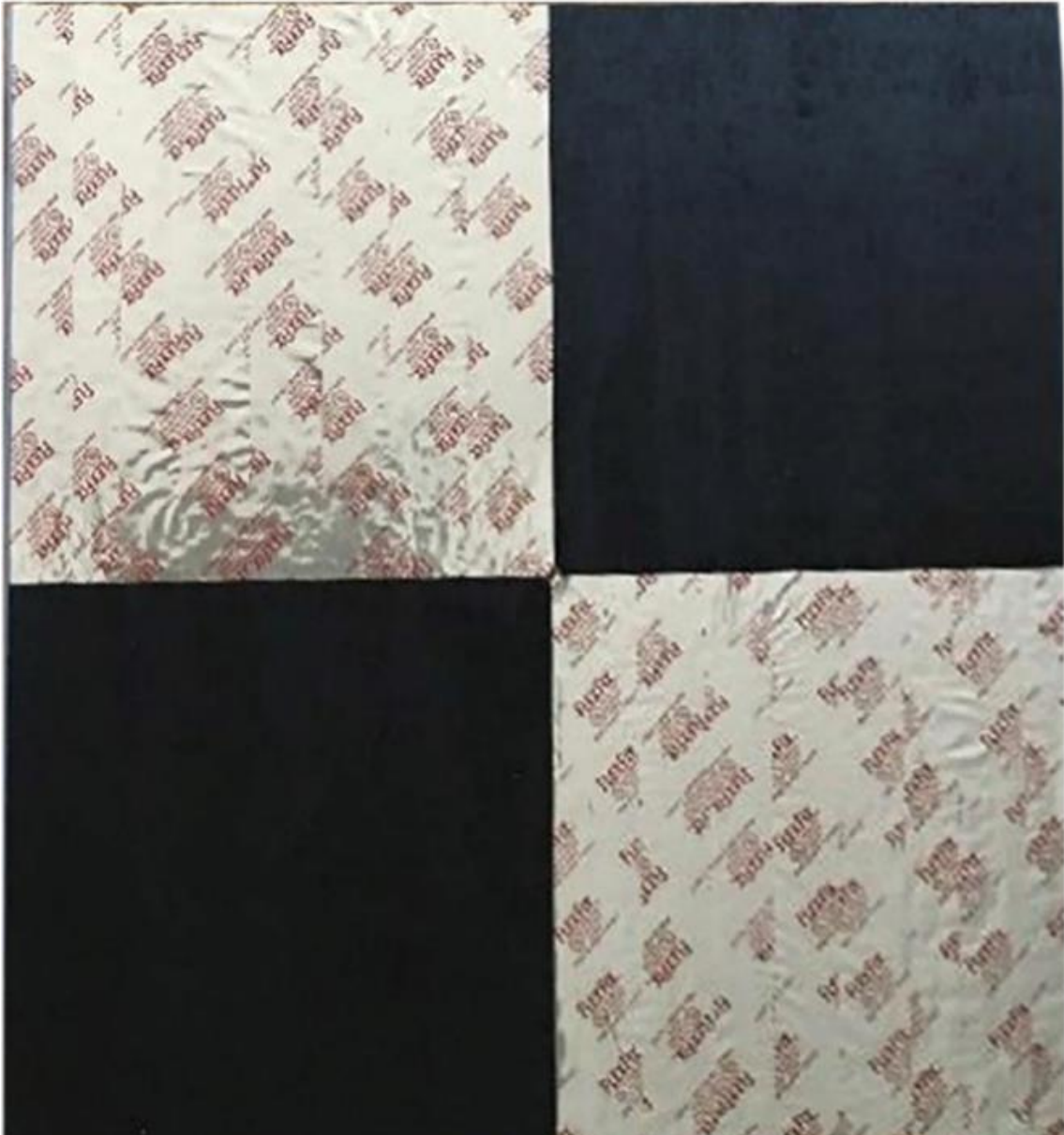
Figure 4.2. Photogrammetric targets were used to ensure accurate georeferencing of thermal infrared orthomosaics. Low emissivity aluminum tape ensured a stark contrast for easy target identification in the thermal images. A small hole was drilled in the center of each target to align it over threaded rod in permanent concrete footers.
