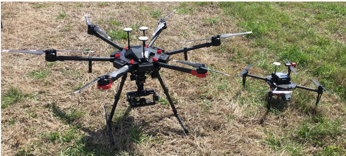
Figure 3.1. DJI Matrice 600 Pro (left) and Matrice 100 (right) with the Infrared Cameras Incorporated 8640P thermal camera and MicaSense RedEdge-3 multispectral camera onboard, respectively.
