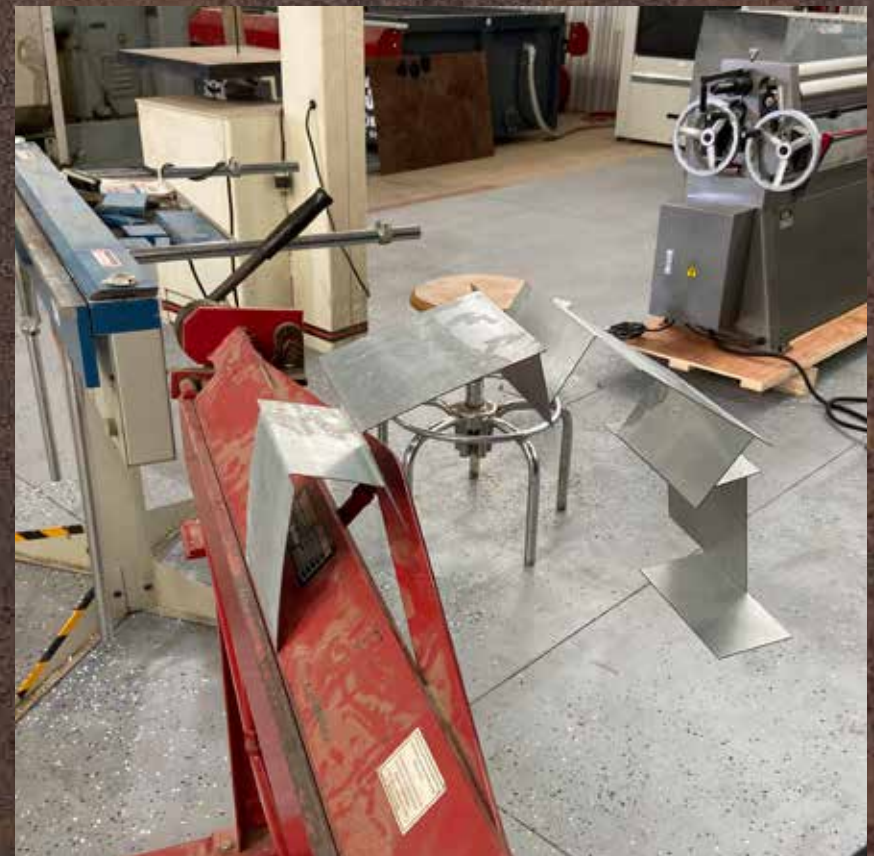
4. Another limitation of the equipment is that it does not allow for 180 degree folds to be fully executed. Because of this, the object starts to create a curved form. After all folds on the finger break are completed, the incomplete folds are finished using pliers to pinch the folds together.
