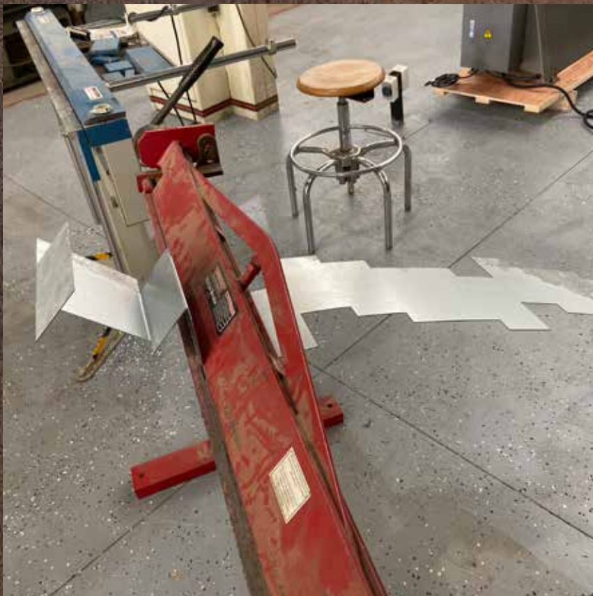
3. Manual finger break used to fold the metal, giving the object three dimensional form. However, due to the limitations of the equipment, the object must be folded starting from one end to the other
