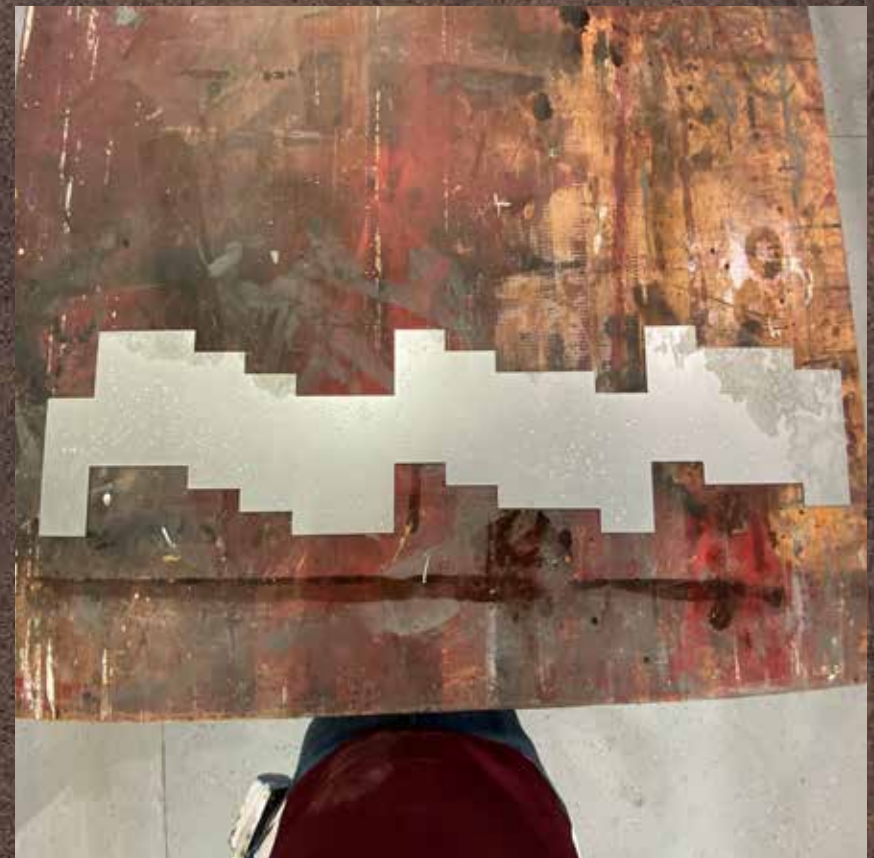
2. Flat shape of object that was drawn on the computer and cut using the water jet.
