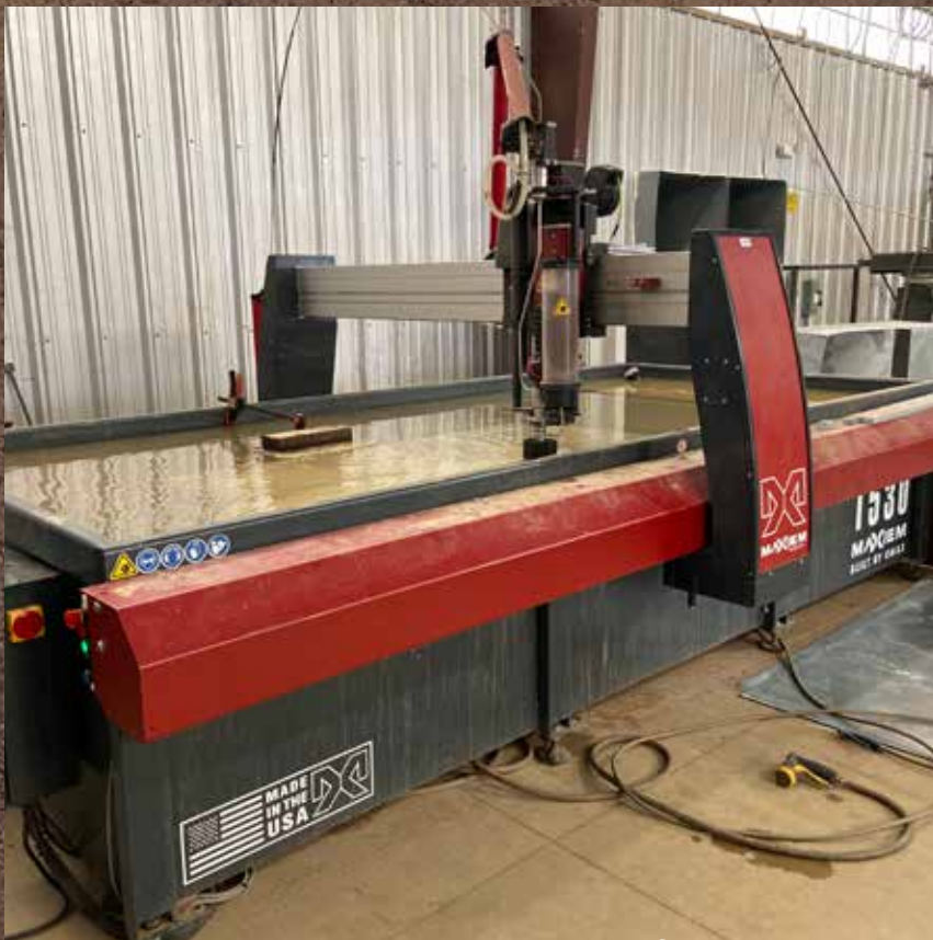
1. Water jet used to precisely cut sheets of metal into desired shape.
