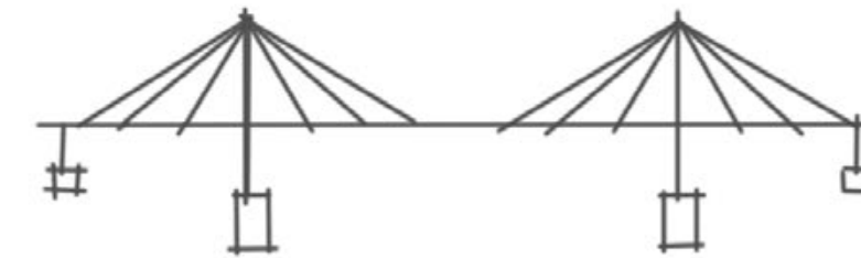
c. Cable Stayed bridge
