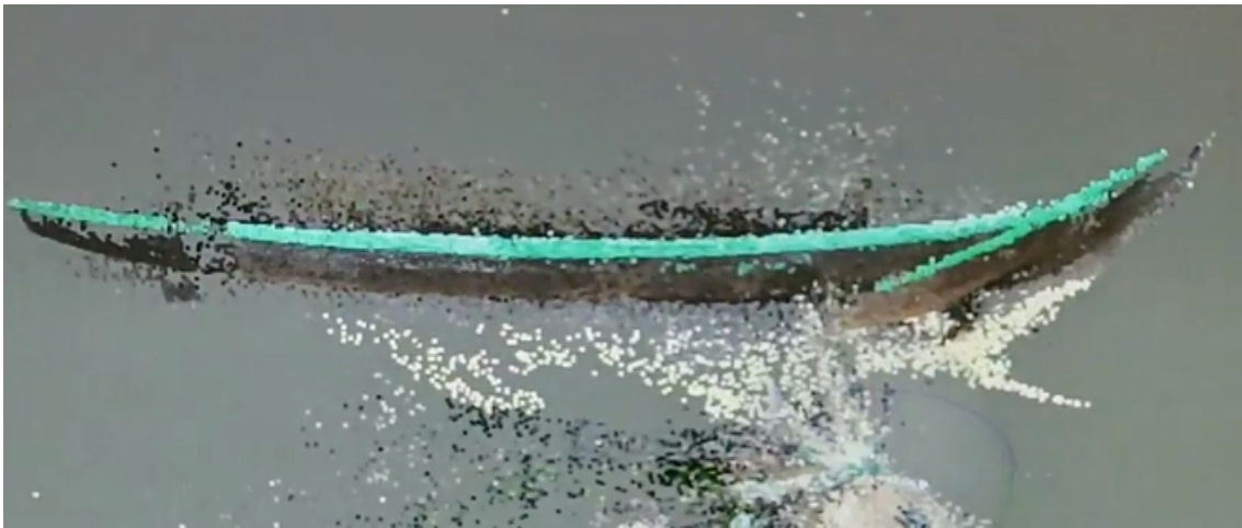
Figure 27: An error in photogrammetric alignment, where two boats were projected at different sizes when there should only be one. Note that the second vessel is the green patch in the cluster of points in the bottom right. Image courtesy of Christopher Dostal, 2019.
