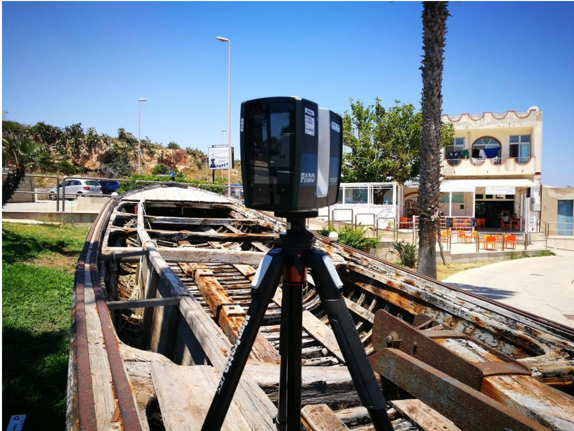
Figure 20: The Faro Focus 3D Laser Scanner used at Portopalo. Image courtesy of the MMHP, 2019.
