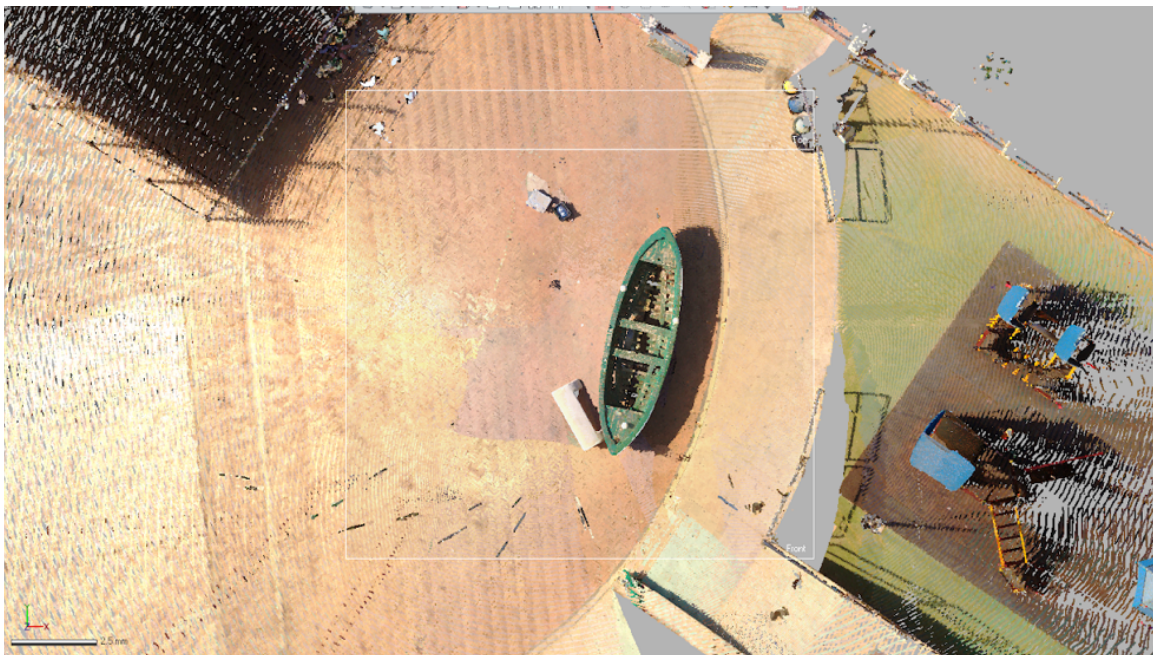
Figure 35: Several laser scans were combined to produce this image. Note the three white spheres on the vessel used to align different scans. © Claire Zak 2020.
