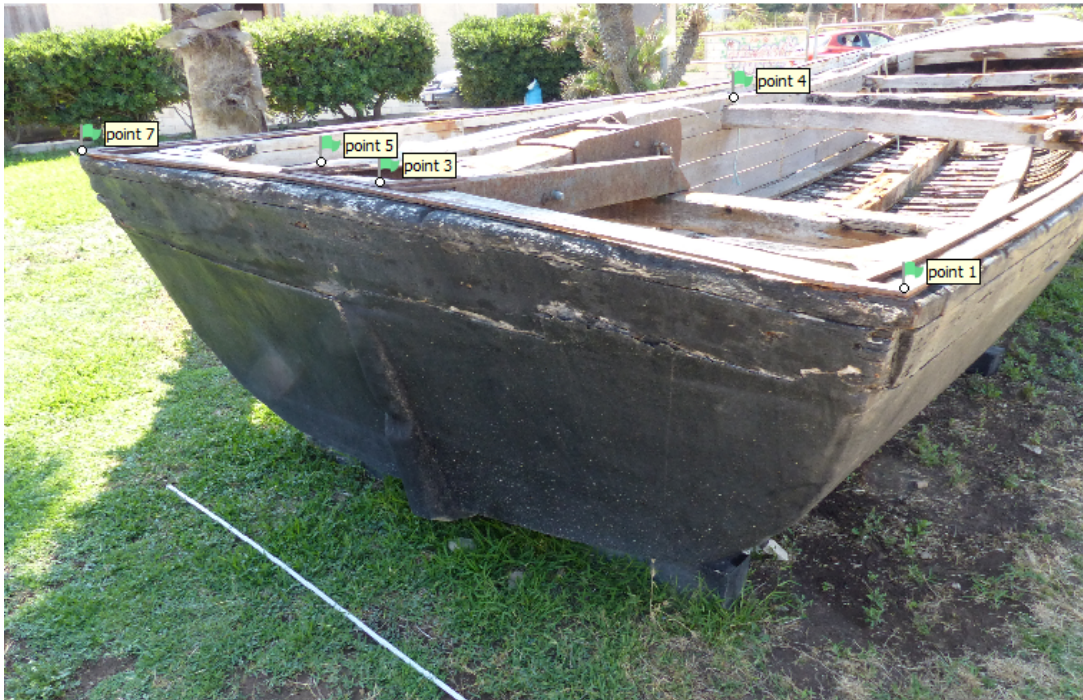
Figure 26: Choosing GCPs is an important step in creating an orthophotograph, which assists in aligning the photographs and georeferencing the model. Image by the author, 2020. © Claire Zak 2020.
