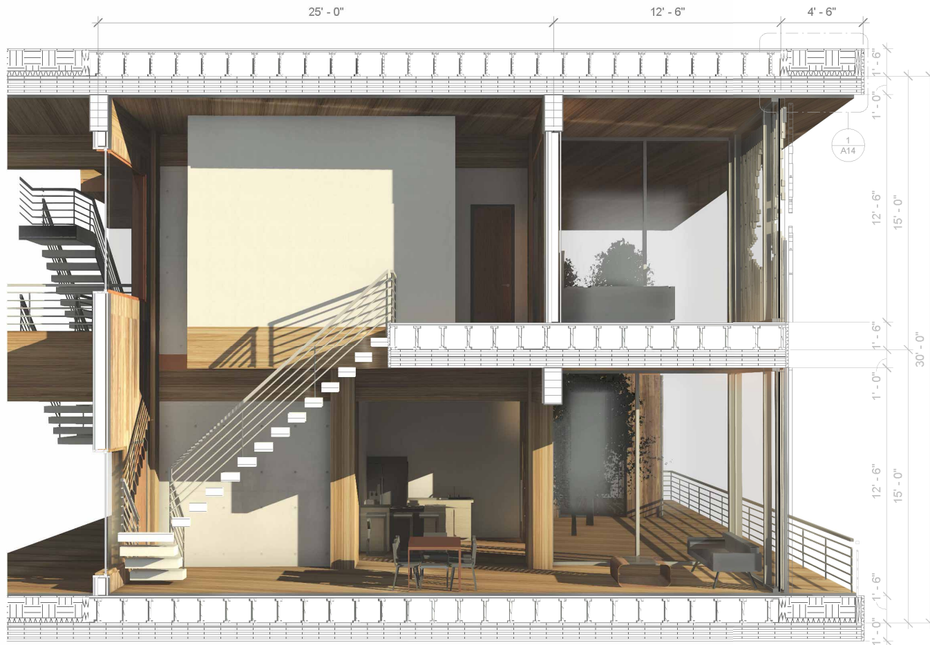
UNIT SECTION B SCALE : 1/2" - 1'-0"
