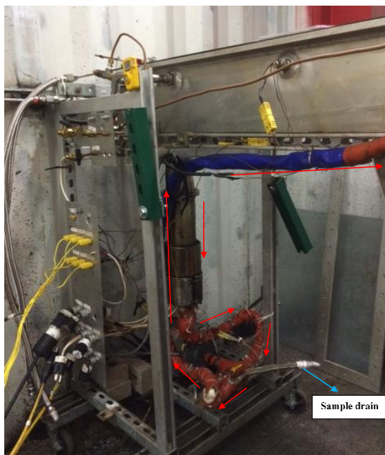
Figure 30: High dose oil irradiation in a flow loop
