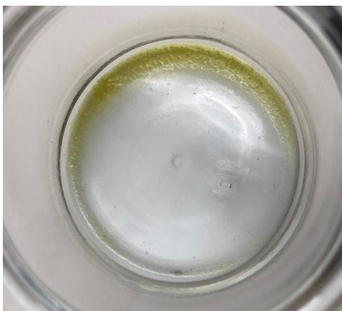
Figure 66: Polymerized benzene due to ebeam irradiation after liquids all evaporated
