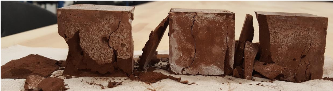
Fig. 4—Crushed cement molds (with Maxcrete).
