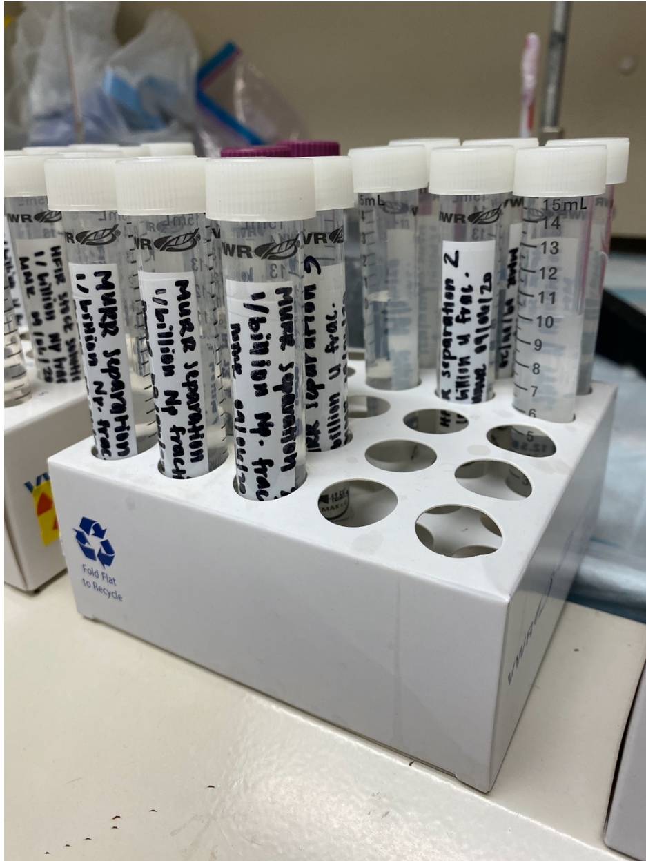
Figure 10. HFIR and MURR samples that underwent single column chromatography prepared for 1 ppb for Np observation and 10 ppb for U.
