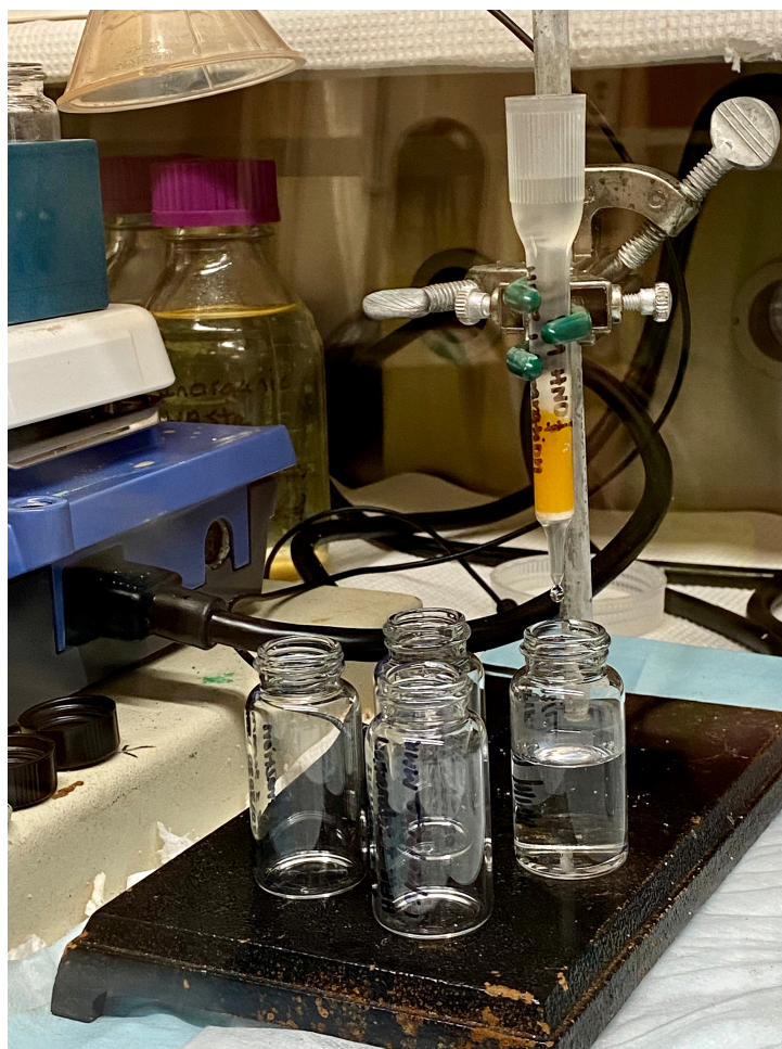
Figure 6. Collection of Pu from the HNO 3 column using 0.01 M HNO 3 .
