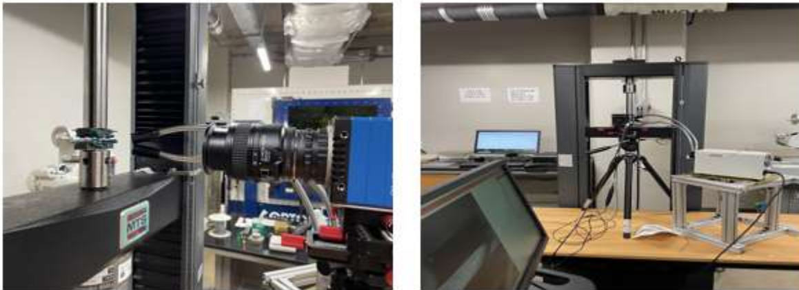
Figure 13. Camera and Lighting setup for DIC.
