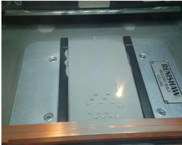
Figure 10. SLM printing using Renishaw AM400
