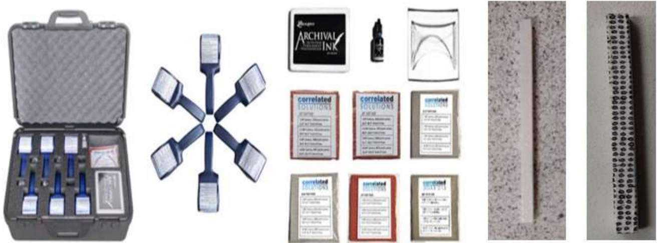
Figure 12. DIC speckling kit and speckled samples
