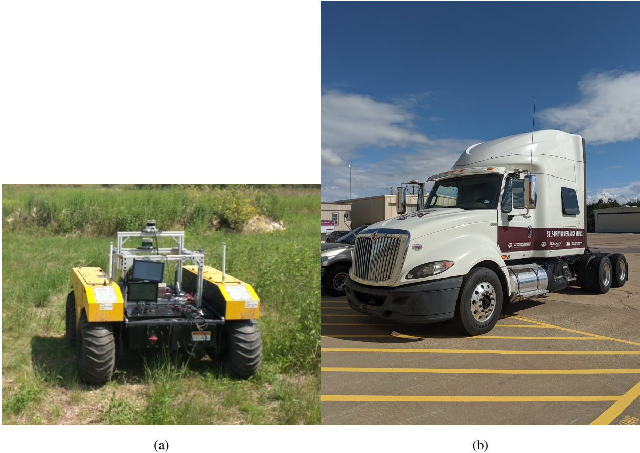
Figure 1.1: (a) Warthog: amphibious unmanned ground vehicle developed by ClearPath Robotics. (b) Autonomous semi-truck in Unmanned Systems Lab, an example of an Ackermann Steering Vehicle .
