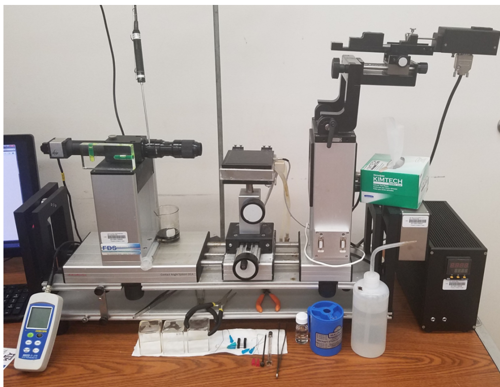
Figure 5.7: All Sessile drop contact angle measurements were performed on the Dataphysics OCA 15 Pro goniometer.
