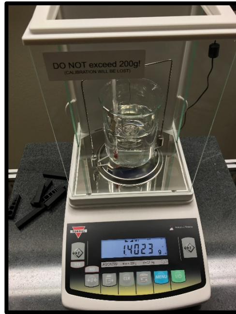
Figure 54. Density test setup based on Archimedes method.
