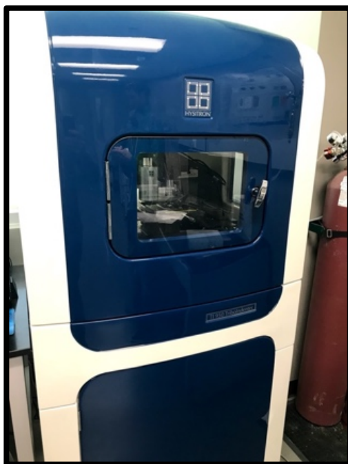
Figure 56. Hysitron TI 950 Triboindenter nanomechanical test setup.
