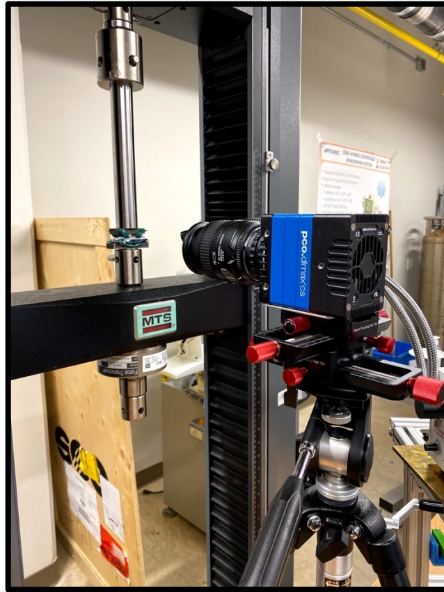
Figure 63. Four-point bending test setup with DIC.
