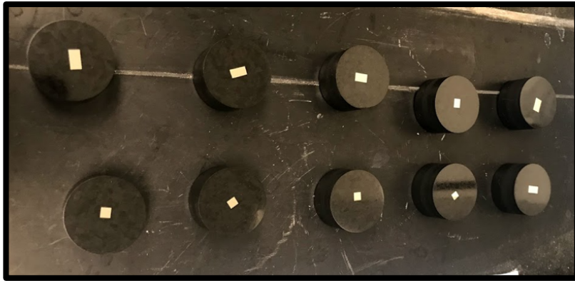
Figure 66. Sectioned and mounted samples in bakelite.
