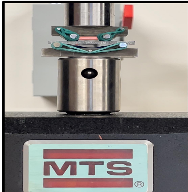
Figure 62. Four-point bending test setup on MTS Exceed test frame.
