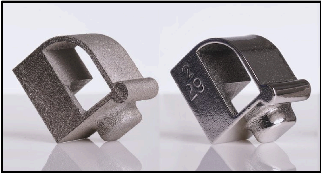
Figure 22. Before and after surface finishing of SS test part [Courtesy: Fintek].
