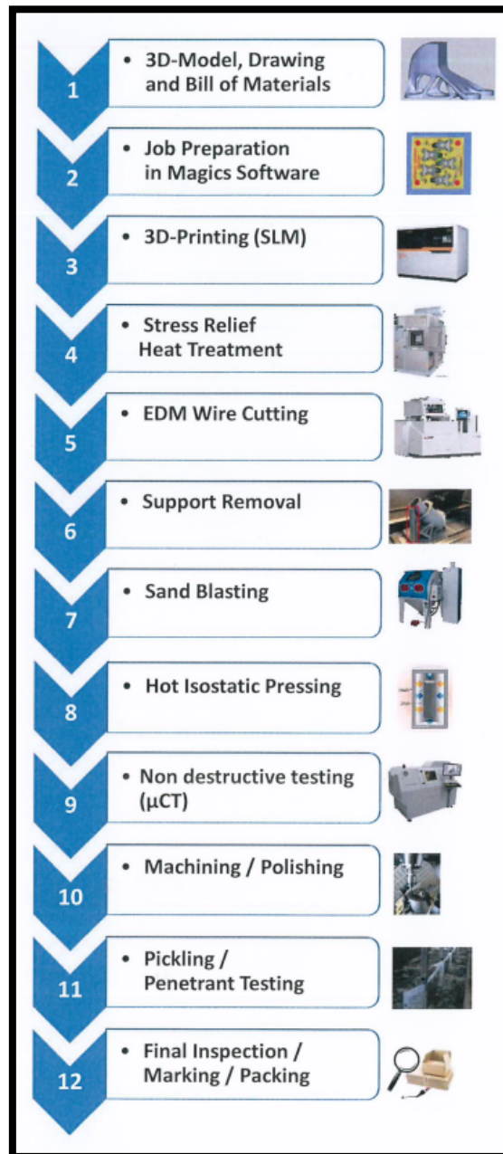
Figure 23. Illustration of steps involved in a typical SLM process [149].
