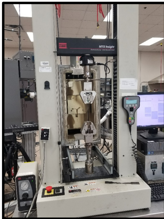
Figure 57. MTS Insight tensile testing setup.
