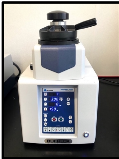
Figure 65. Buehler SimpliMet 4000 mounting press.
