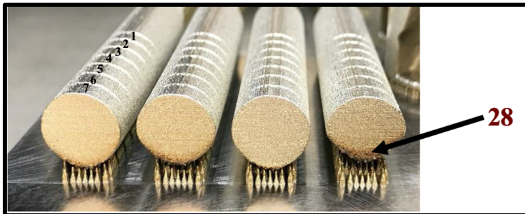
Figure 72. As-built samples on the build plate with the support structures. Sample numbers are also indicated. Observe that sample #28 exhibited curling due to higher energy input.
