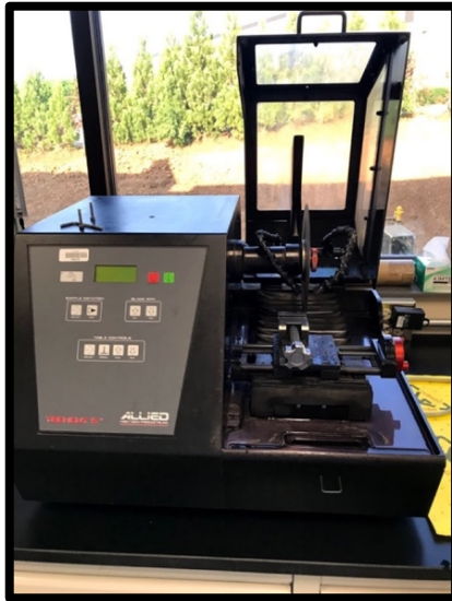
Figure 64. Allied TechCut 5 precision saw to section specimens.
