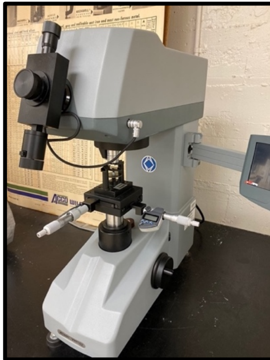
Figure 55. Beuhler Wilson VH1102 microhardness tester.
