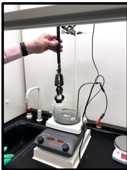
Figure 68. Electrochemical etching setup.
