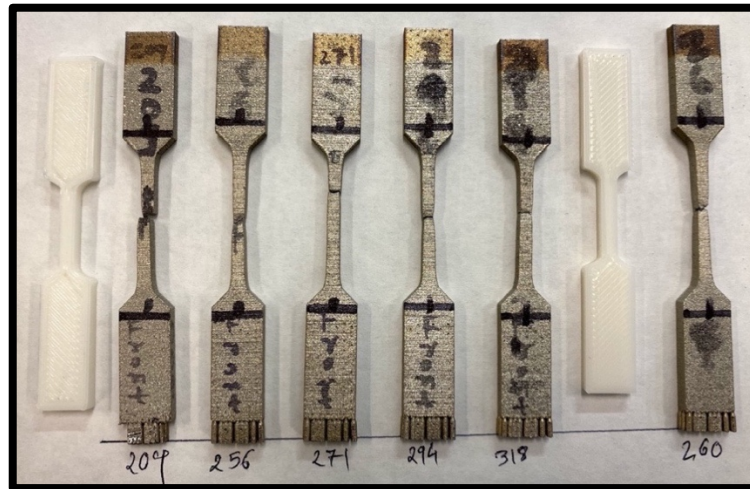
Figure 137. Side by side comparison of fracture location in the gauge section of front tensile samples.
