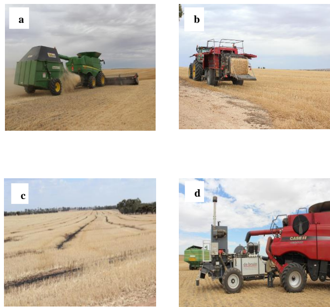
Figure 3. Examples of harvest-time weed seed management tactics practiced in Australia: a) chaff cart, b) bale-direct system, c) narrow-windrow burning, and d) Harrington Seed Destructor (photo credit: MJ Walsh, AHRI)
