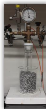
Hydrogenation: 75 psig of \text{H}_2 @ 375 °C for 30 min
