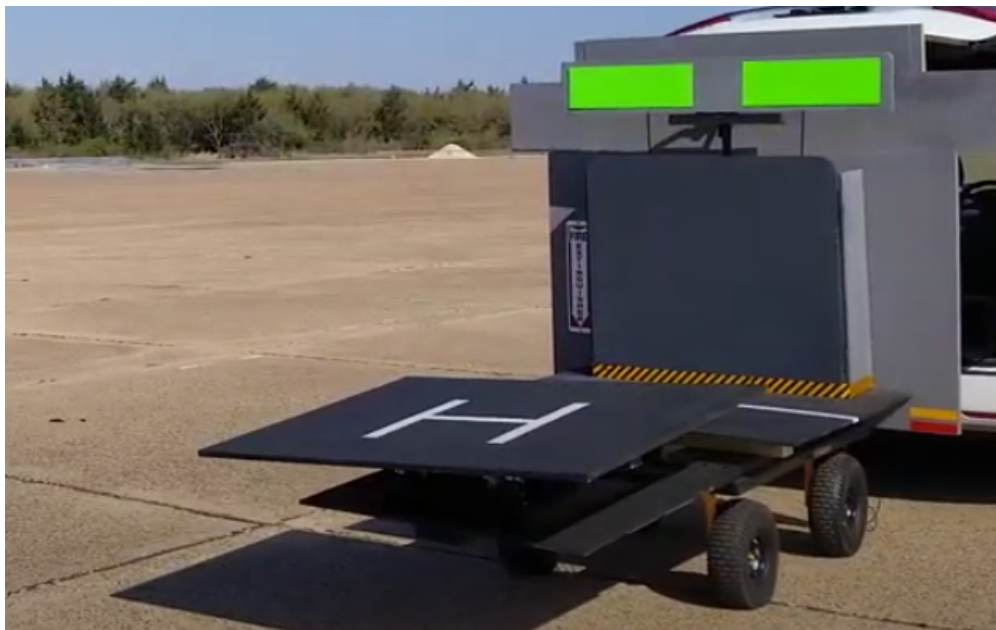
Figure 5.6: Constructed ship platform with horizon bar and motion deck
