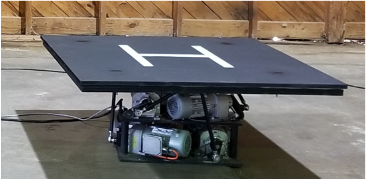
Figure 5.2: Servos and Simulation Inc. 6 DOF motion system with 4 ft x 4 ft landing deck
