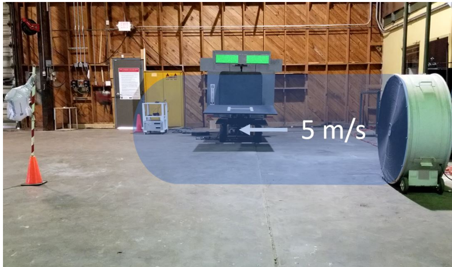
(a) Crosswind testing setup
