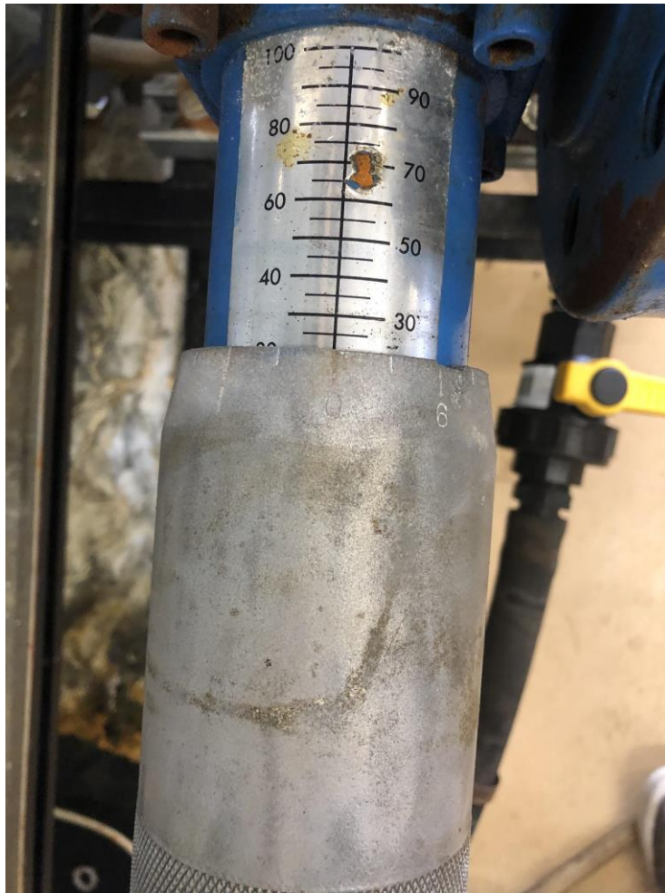
Figure 21. Dial on the pump used to control capacity
