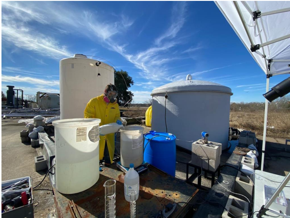
Figure 28. Proper PPE while adding acid to inlet tank
