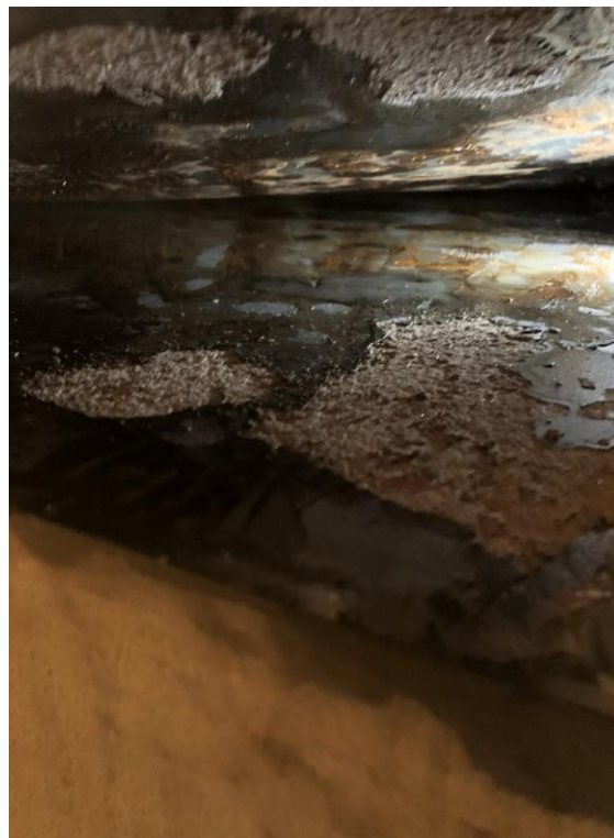
Figure 18. The plate (top) and the block (bottom) when pulled apart
