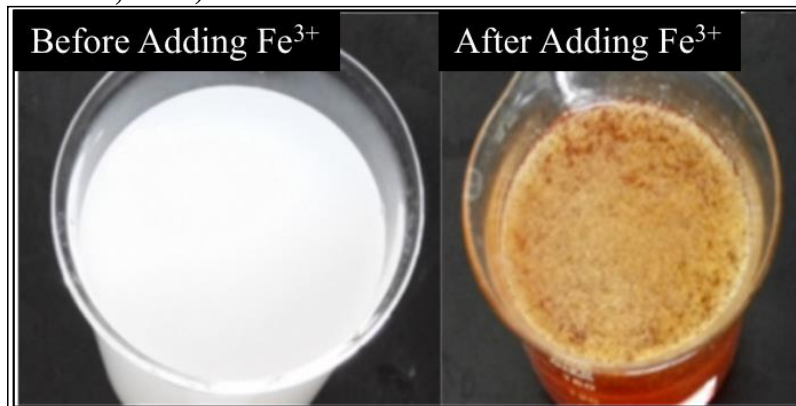
Figure 6: Effect of Fe^{3+} on the Flocculation of Friction Reducer Molecules (Wu et al., 2017). Fe^{3+} is from the common mineral pyrite in the shale formation.
