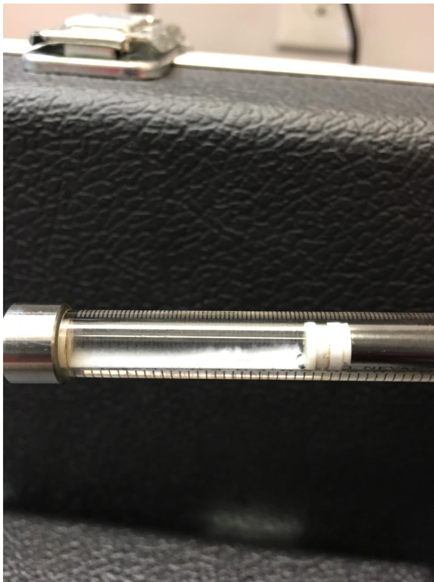
Figure 45: Precipitation in the micro viscometer from LDFR solution with \text{CaCl}_2 .
