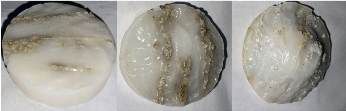
Fig. II-16 Marble disks from RDA experiments performed at 150°F using 15 wt% HCl and 1 wt% corrosion inhibitor. The disks rotational speeds from left to right were 132, 584, and 1,172 rpm. Reprinted with permission from (Kotb and Nasr-El-Din 2020).
