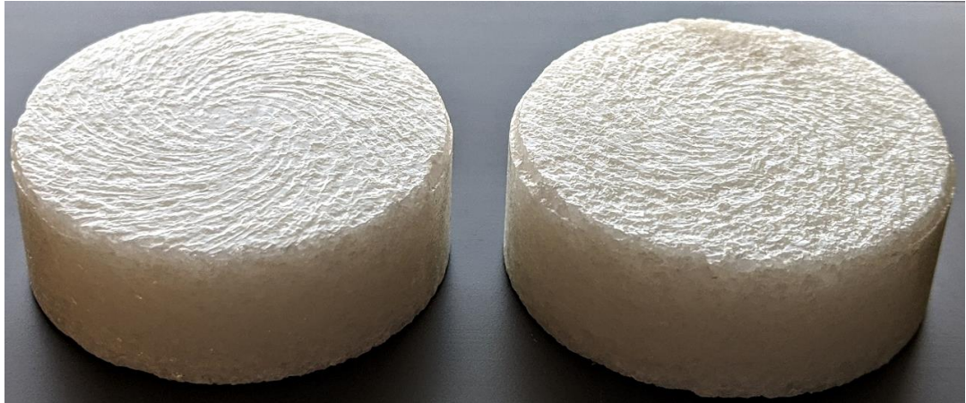
Fig. III-11 1.46 in. disks composed of grains of maximum size of 1000 \mu\text{m} after dissolution in 1N HCl at 73.4°F, and disk rotational speeds of 518 (left) and 1,175 (right) rpm. Reprinted with permission from (Ivanshin et al. 2021).
