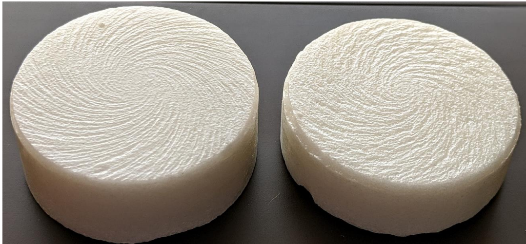
Fig. III-12 1.46 in. disks composed of grains of maximum size of 150 \mu\text{m} after dissolution in 1N HCl at 73.4°F, and disk rotational speeds of 518 (left) and 1,175 (right) rpm. Reprinted with permission from (Ivanshin et al. 2021).
