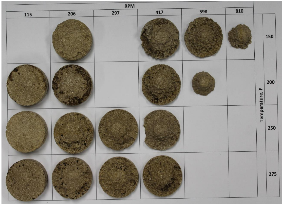
Fig. IV-11 Indiana limestone disks after the RDA experiments. Reprinted with permission from (Kotb et al. 2021).
