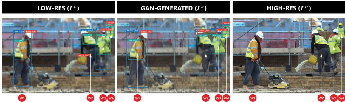
Figure 36. An example of object detection by YOLO-WHV for low-resolution ( I^L ) and GAN-generated ( I^S ) images with an input size of 96 \times 96 .
