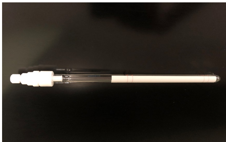
Figure 7: Falling Ball Viscometer
