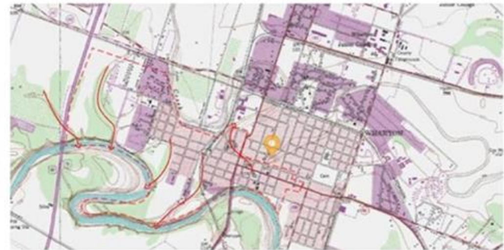
By the USGS Classic Quad Map (terrain and contours 2016), Get the predicted drainage flow direction in planning zone.
