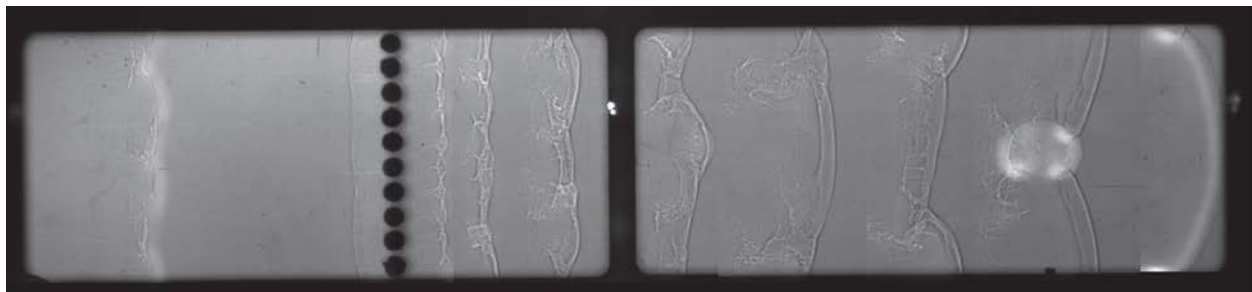
Figure 8: Overlay of multiple shadowgraph video frames showing the evolution of the wave front in an ethane-oxygen mixture at p_0 = 3.4 kPa (0.5 psi).
