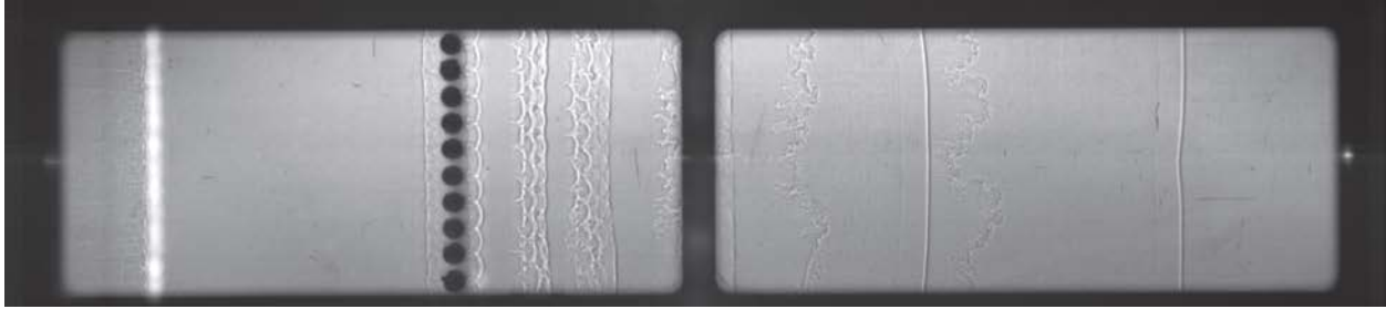
Figure 13: Overlay of multiple shadowgraph video frames showing the evolution of the wave front in an acetylene-oxygen-argon mixture at p_0 = 9.6 kPa (1.4 psi).
