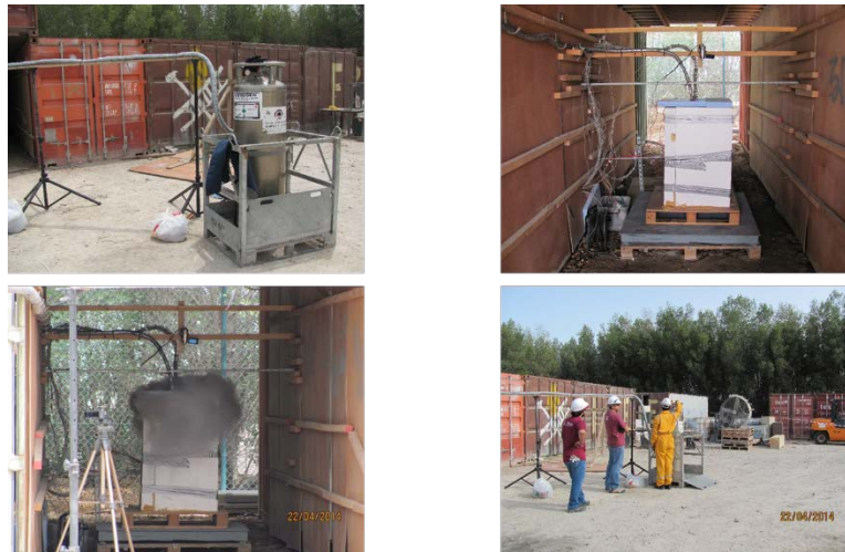
Figure 3: Liquid nitrogen and liquid oxygen spill over concrete experiment at RLIC
