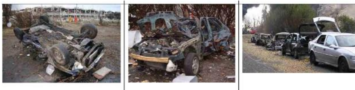
Figure 10. Vehicle damage and vegetation proximity at the Buncefield site – Courtesy HSE UK Report
