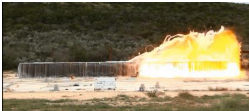
Figure 6. BakerRisk Vapor Cloud Explosion Test Rig – Courtesy BakerRisk
