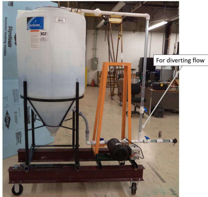
Figure 15. The custom-made frame that hold 110-gallon mixing tank, flow pump, VFD, flow sensor, and flow diverting line on the wheels.
