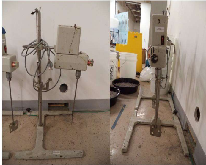
Figure 17. CARFRAMO RZR50 Fluid Mixer used to mix the guar with water.
