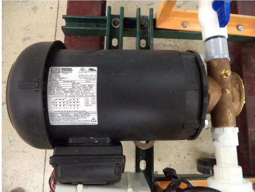
Figure 11. WEB brand general motor with \frac{3}{4} hp that can pump at 21 gpm with 10 % solid contents
