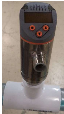
Figure 13. Flow meter to measure the flow rate in real-time and post experiment.
