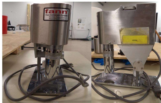
Figure 18. FANN Viscometer used to measure viscosity of the test fluids.
