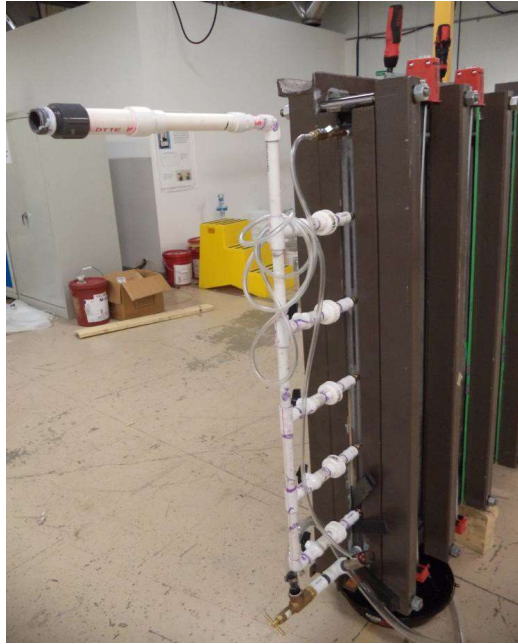
Figure 9. Inlet pipe setup showing five inlets with valves, pressure sensor on bottom and fluid bleeding valve at the top.
