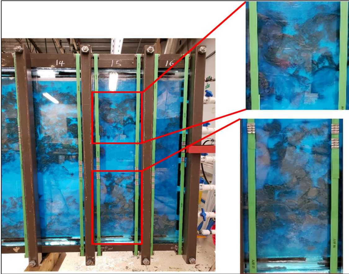
Figure 52. Fiber-proppant-flocculation showing the random suspended islands. (0 wt. % guar, 0.3 wt. % PGA (13 mm), 30/50 ceramic proppant).
