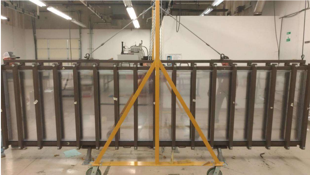
Figure 8. Large apparatus assembly with crane to hold the frame upright.
