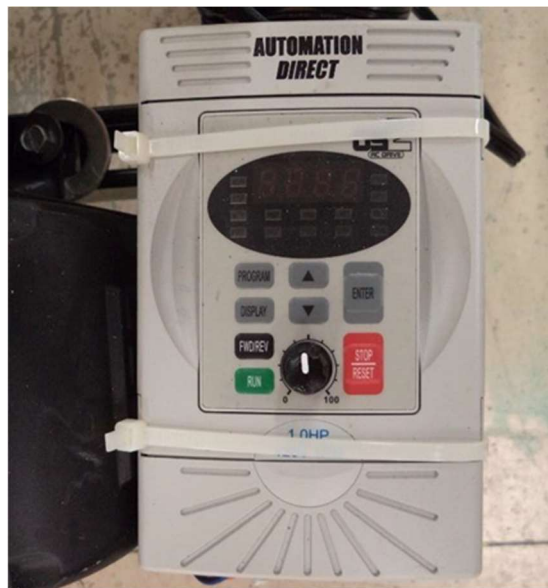
Figure 12. The variable frequency drive used to control the flow rate of the pump
