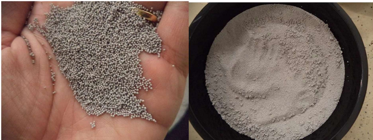
Figure 21. The 20/40 mesh ceramic proppant with 2.69 g/cc density used for experiment.
