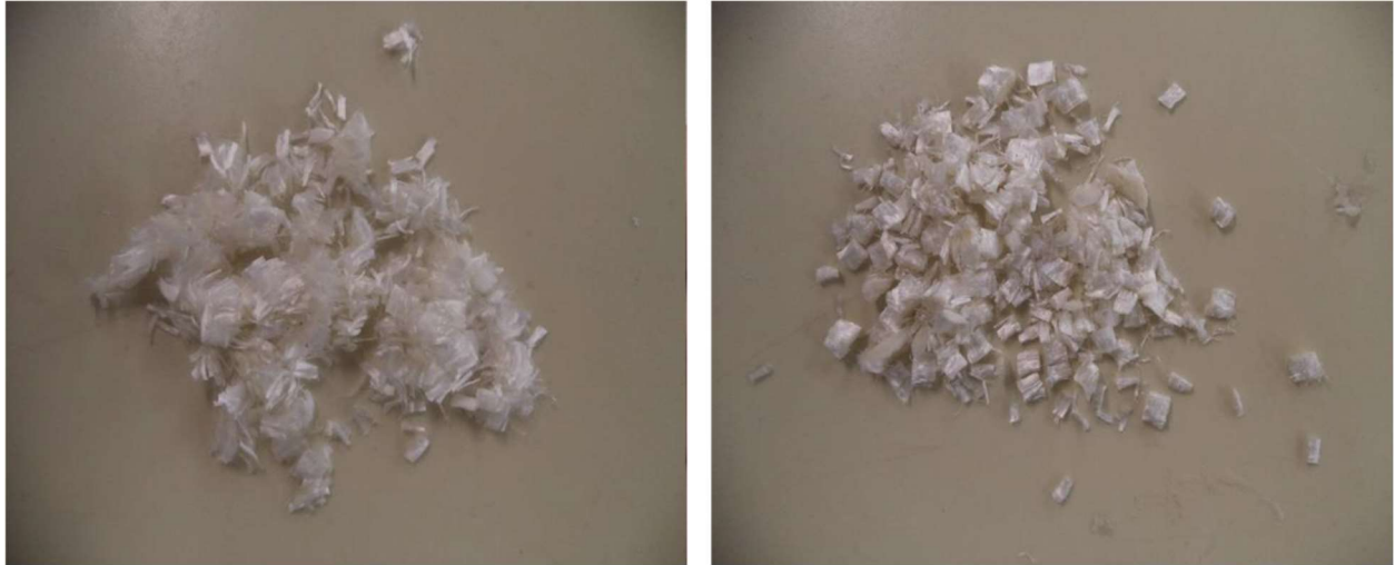
Figure 22. The fibers used for experiment (PGA fiber on left and PLA fiber on right).
