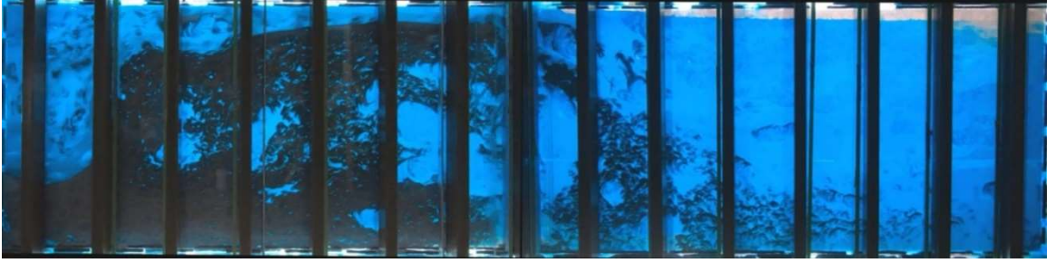
Figure 39. Proppant transport without guar at 2 minutes of pumping the slurry shows channel formation acting as a flow conduit for following slurry to flow through (0.3 wt. % fiber (PGA 13 mm), 40/70 ceramic proppant, 1.8 cp).
