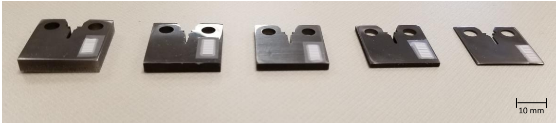
Figure 3.3. A set of NiTi CT specimens with nominal thickness values from 1mm to 5mm (from right to left)
