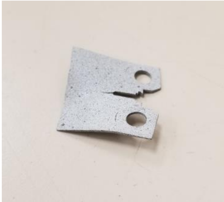
Figure C.2. Photo of the sample having 1 mm thickness buckled at the end of the fracture experiments
