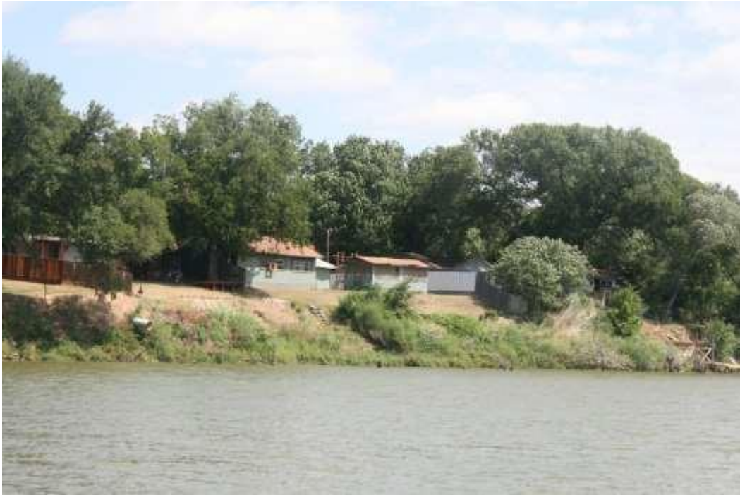
Figure 172: Modification typically included vegetation removal, structures built close to the river channel, and little or no stabilization.
