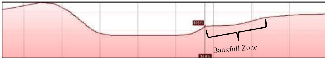
Figure 60: Example of bankfull zone: region extending from threshold of main channel and step wide enough to sustain permanent structures, and the threshold of the main floodplain.
