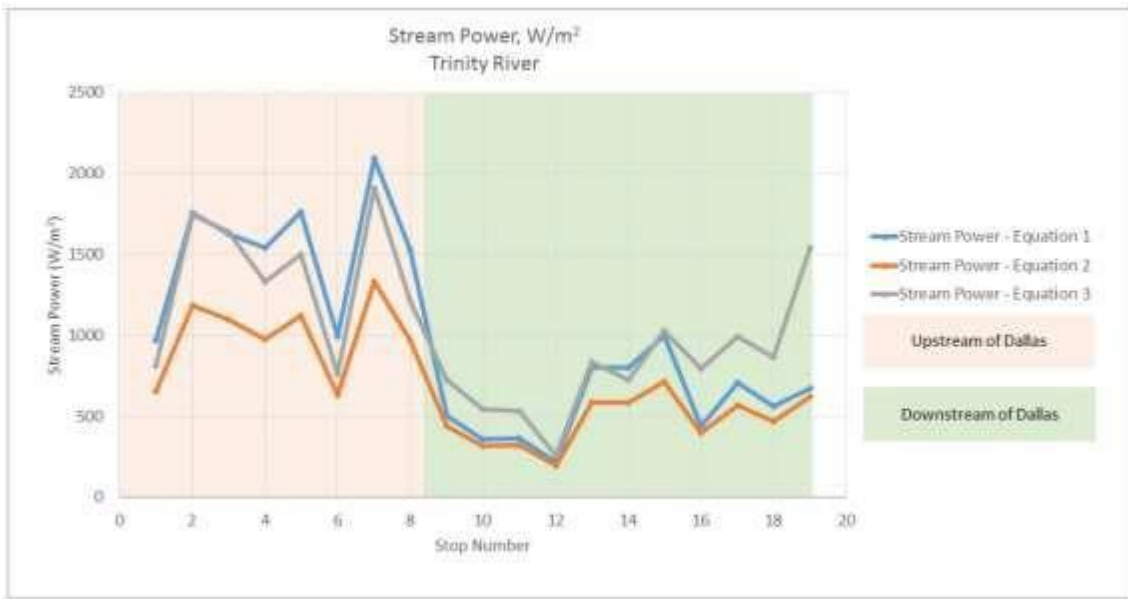
Figure 18: Values for stream power ( W/m^2 ) for the Trinity River near Dallas, Texas.
