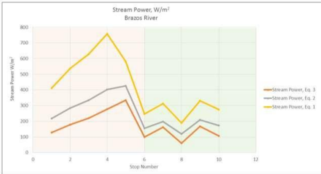
Figure 15: Stream power values, Brazos River near Waco. Red background indicates stops upstream of Waco and green background indicates stops downstream of Waco.
