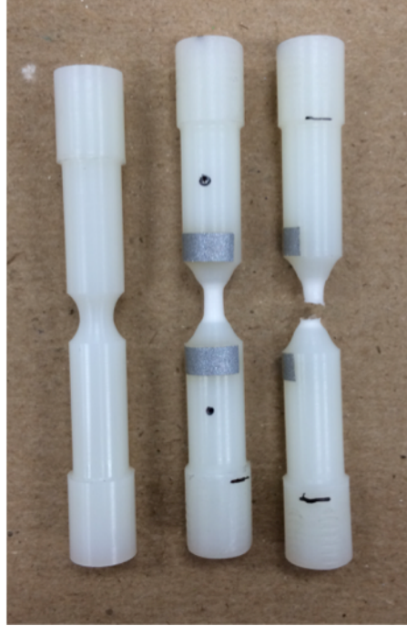
Figure E.2: (Left) An undeformed RN10 bar used in preliminary studies. (Middle) An RN10 bar of PA-6 loaded and interrupted immediately prior to fracture. (Right) An RN10 bar of PA-6 loaded to fracture. Both tests were carried out at room temperature ( 24^{\circ}\text{C} ), with a nominal strain rate of 10^{-3} /s, and 217 days after receipt of the raw material.
