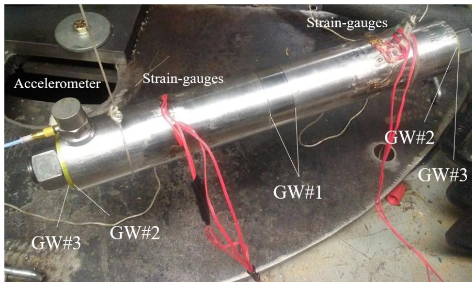
Figure 3.5 Photo of the strain gage instrumented, axially preloaded test shaft
