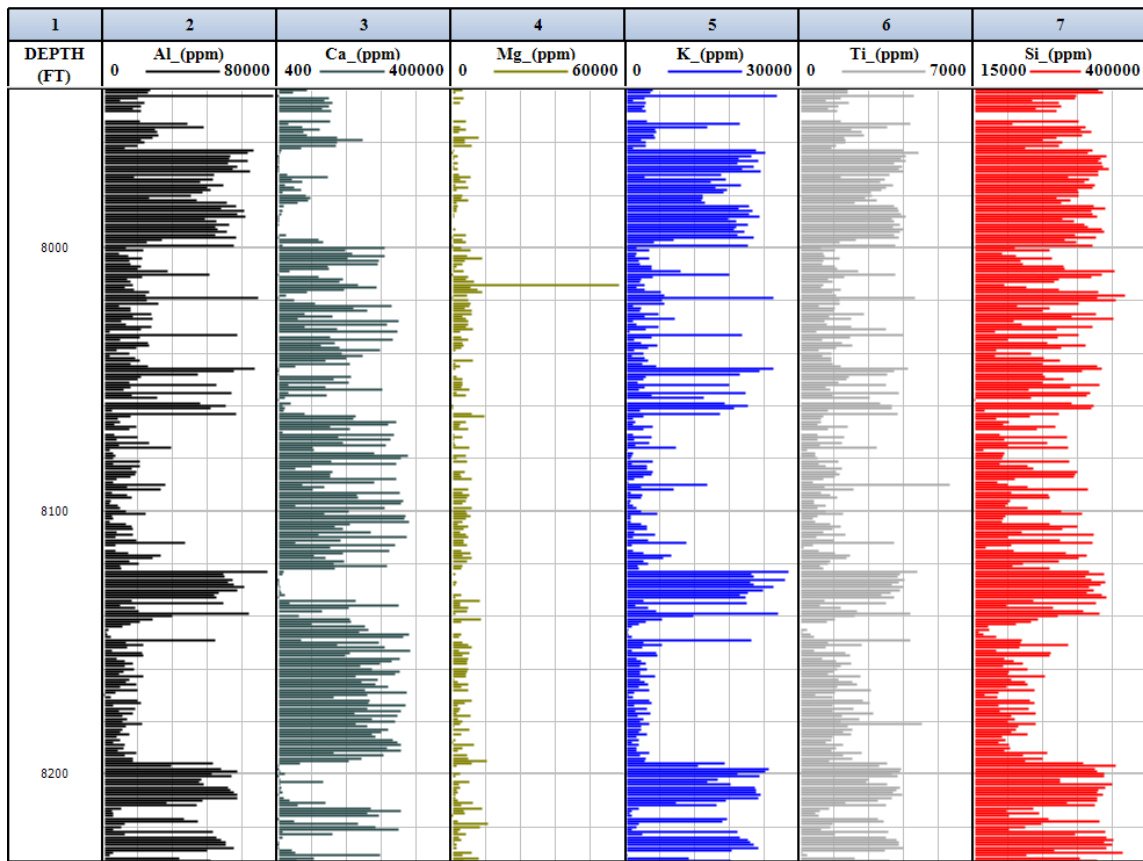
Figure V-3: Elemental Composition from XRF (X-ray Fluorescence) spectroscopy for select elements: Aluminum (Track 2), Calcium (Track 3), Magnesium (Track 4), Potassium (Track 5), Titanium (Track 6) and Silicon (Track 7)
