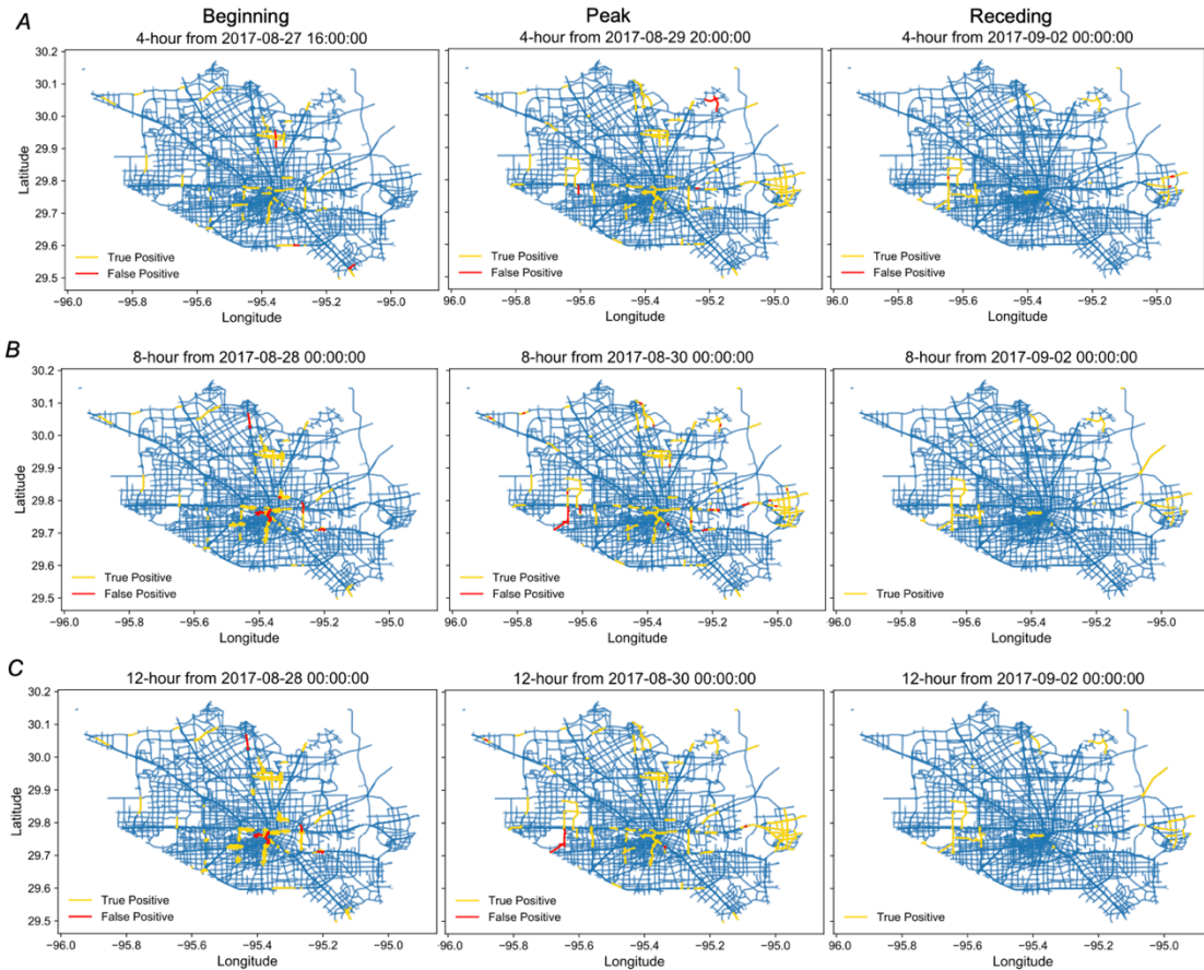
Figure 17 Examples of three prediction models for different phases of the flooding period (i.e., propagating, peak, and receding phases). (A) the model for predicting the situation in next 4 hours; (B) the model for predicting the situation in next 8 hours; and (C) the model for predicting the situation in next 12 hours. The true positive (yellow) and false positive (red) road segments are all actual flooded road segments from the empirical INRIX data in a specific time interval.
