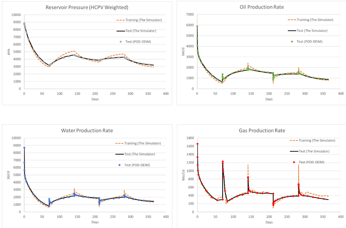
Figure 3.26 Comparison of the performance of training and case 3. Results of the POD-DEIM application show strong match within less than 0.1% error. Reprinted with permission from SPE-198946-MS.
