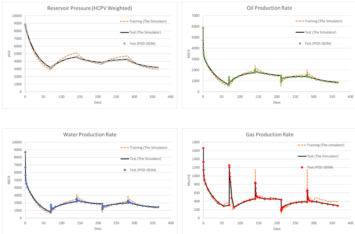
Figure 4.9 Comparison of training and test case 2. The performance of the POD-DEIM with ANN model shows an excellent match to the full-order simulator.
