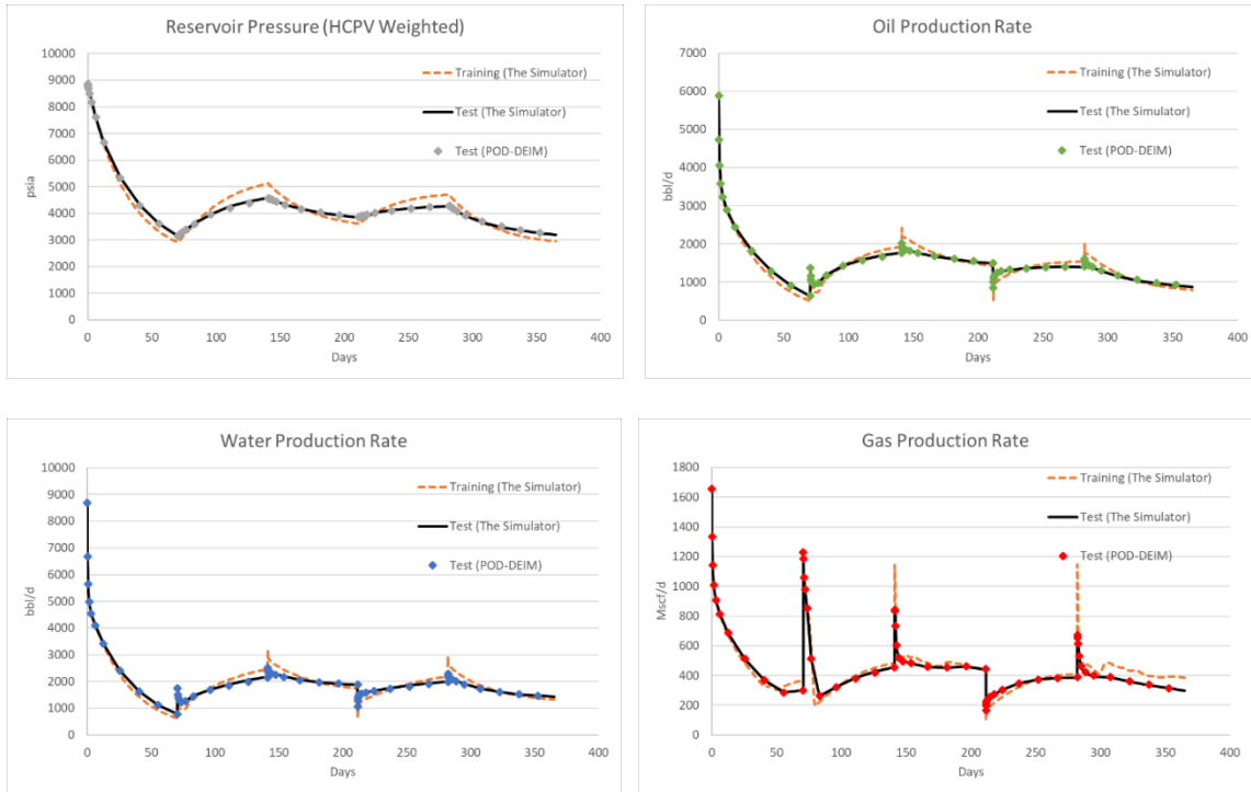
Figure 4.12 Comparison of training and test case 3. The performance of the POD-DEIM with ANN models shows a strong estimation with less than 0.1% error.
