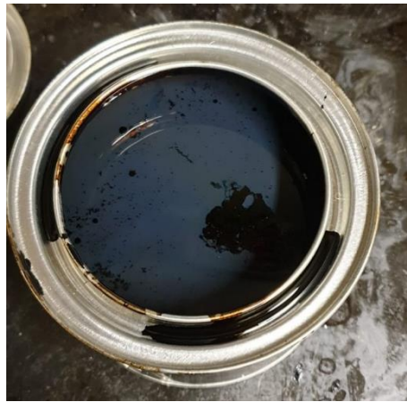
Figure 22: White PE wax film on the modified asphalt binder.
