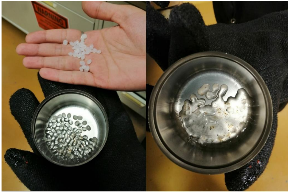
Figure 46: White opaque pellets of LDPE 4, as received, and the translucent pellets after a short period of heating.
