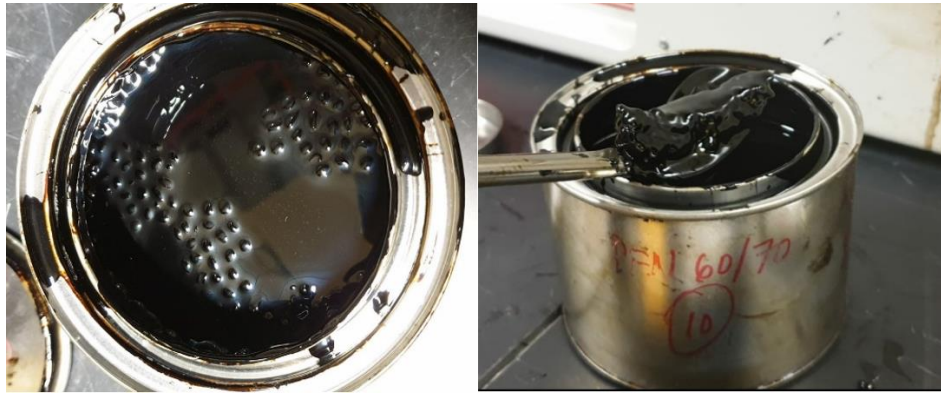
Figure 45: Solid LDPE 4 pellets phase separating from the binder
