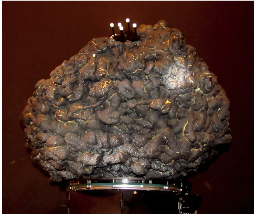
Figure 6.22: The mock asteroid placed on the turn table. The VICON dots can be observed placed at the top on a mounting plate. Reprinted with permission from [55].
