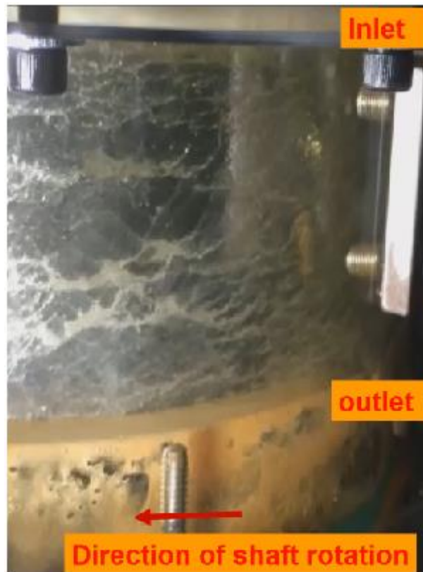
Figure 2 Flow visualization of wet seal operating with a gas and oil mixture. Inlet GVF = 0.9, journal speed = 1,800 rpm. Pictures taken with a stroboscope light at 30 Hz. Seal inlet pressure ( P_s ) = 2.0 bar (a), discharge pressure ( P_a ) = 1 bara. Picture reproduced from Ref. [11]. The author of this dissertation holds the copyright of Ref. [11].
