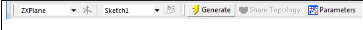
Figure F.16: Top panel where the “Generate” feature is found to validate a design description
