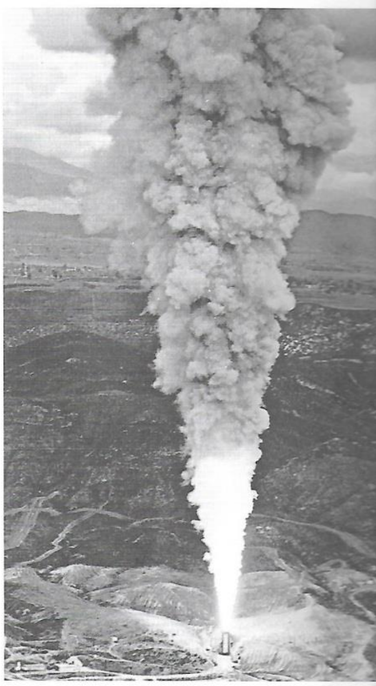
Figure 2.1: High Reynolds number turbulent jet produced by the test of a rocket by Lockheed in Redland, CA. Reprinted from Lockheed Martin, 1968
