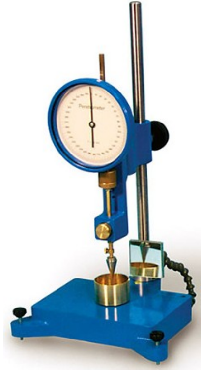
Figure 3 Picture of the fall cone apparatus.
