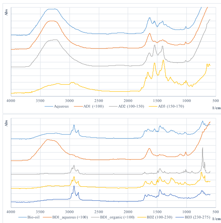
Figure 4.11. FTIR spectra of aqueous and bio-oil distillate fractions.
